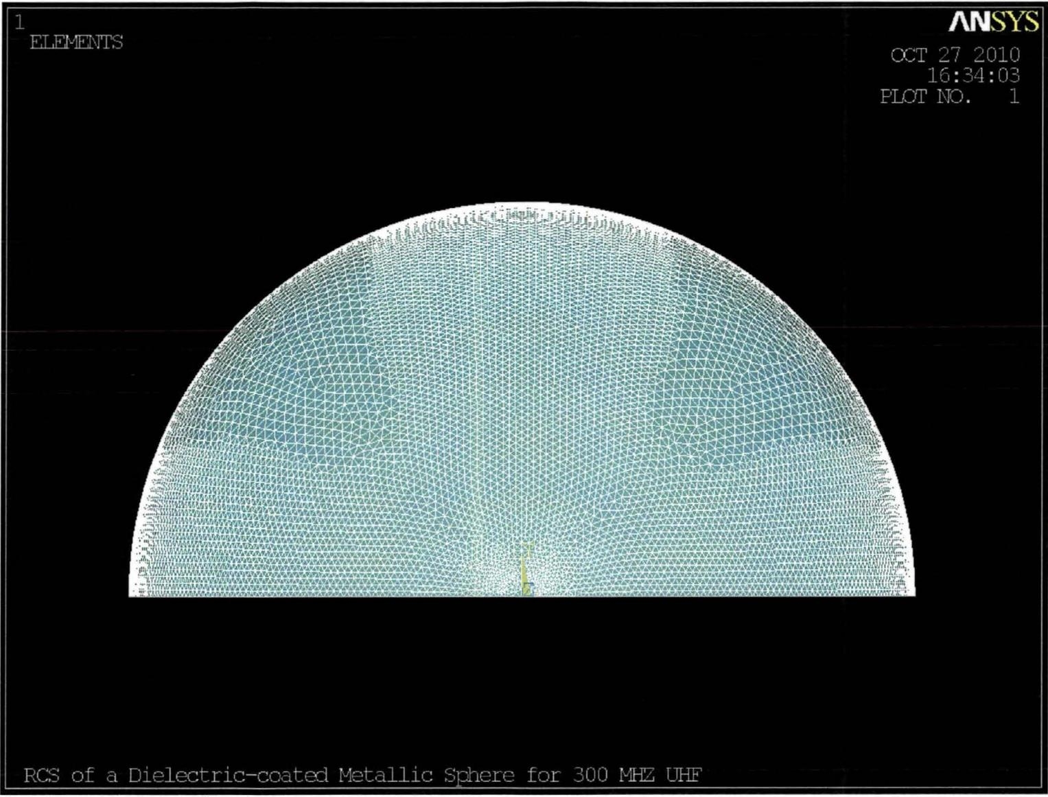
Figure 61. Mesh of 1/2 Symmetry UFO Sphere with 50 Elements per Wavelength
